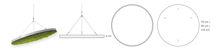
Technical Specification **GL-C-115** Glade Ceiling Large Width: Ø115 cm Thickness: 4 cm Weight: 8.6 kg
